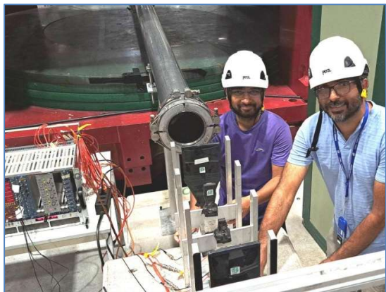
Students from SINP setting up beam scintillator in CERN HGCal test beam 2023.
