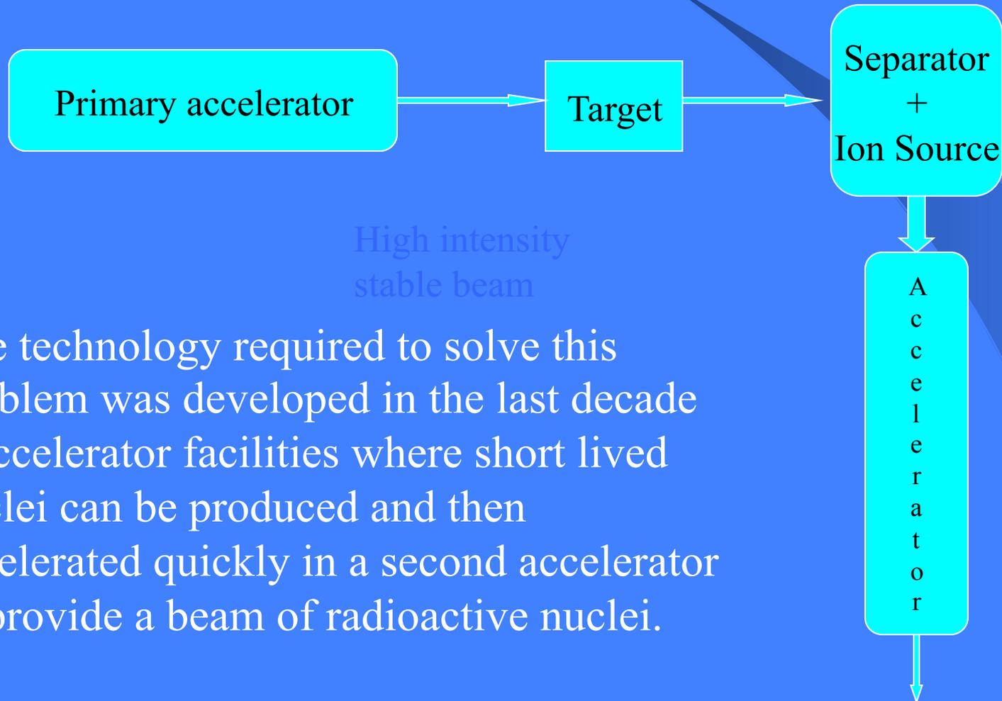
The technology required to solve this problem was developed in the last decade – accelerator facilities where short lived nuclei can be produced and then accelerated quickly in a second accelerator to provide a beam of radioactive nuclei.
